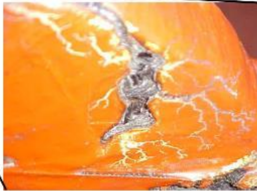
Insulation Damage from Electrical Tracking
